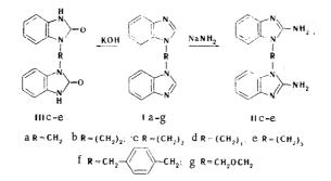
Compounds Ia, b, f, g do not react with sodium amide in xylene solution, while a reaction accompanied by the evolution of gases ( $CO_2$ ,  $NH_3$ ,  $H_2$ , and hydrocarbons) is observed in dimethylaniline. Only in the amination of If were we able to isolate 25% of the starting compound and 13% of the benzimidazole. Compounds Ia, b,
